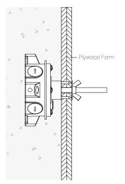
6" (152mm) threaded rod is supplied. Thread size: 3/8"-16
