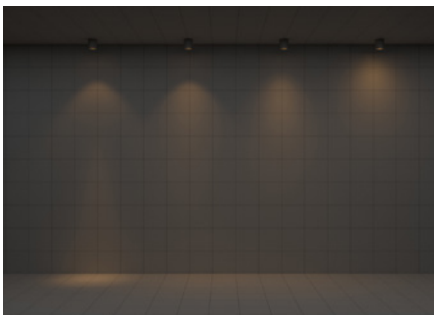
Left to right: 10° (Spot beam), 30° (Narrow Flood), 40° (Flood beam), 60° (Wide Flood beam)
