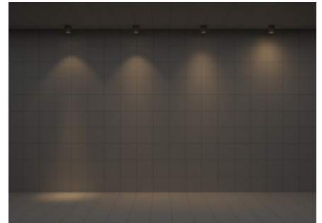
Left to right: 10° (Spot beam), 30° (Narrow Flood), 40° (Flood beam), 60° (Wide Flood beam)
