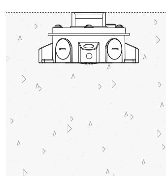
Fixture inserted: Complete Concrete Installation
