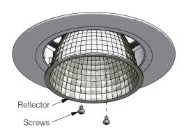
Once reflector is removed grip trim firmly and pull down.
