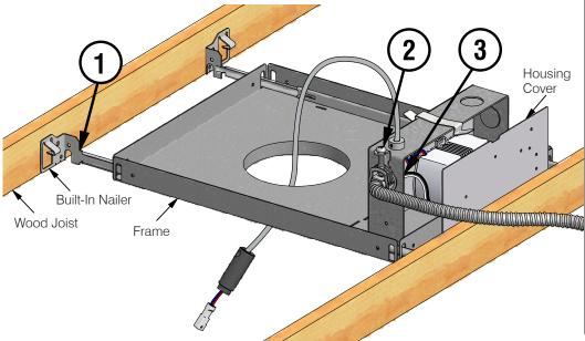
\*Do not use lamp holder / LED trim unit as temporary lighting. Plug-in connector cannot support weight of hanging LED Unit.
