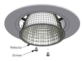
Replace with new LED Zhaga Module and reverse the steps.
