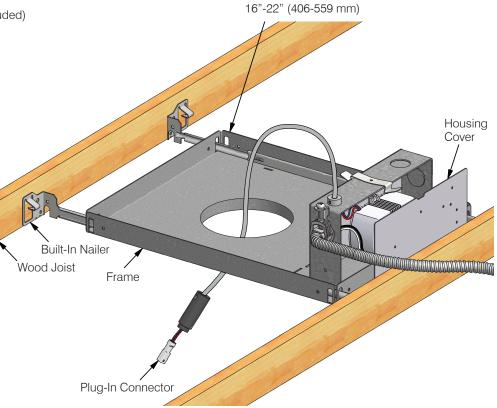
\*Do not use lamp holder / LED trim unit as temporary lighting. Plug-in connector cannot support weight of hanging LED Unit.
