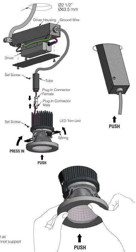
\*Do not use lamp holder / LED trim unit as temporary lighting. Wire connection cannot support weight of hanging LED Unit.
