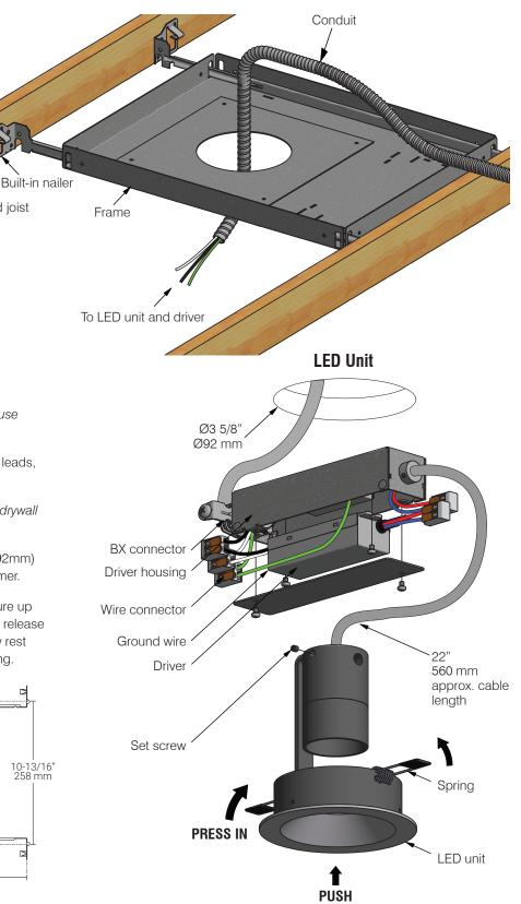
\*Do not use lamp holder / LED trim unit as temporary lighting. Wire connection cannot support weight of hanging LED Unit.
