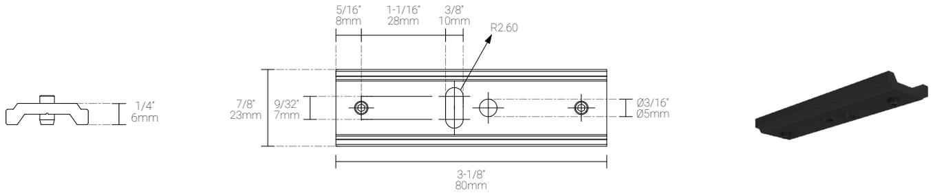
**1CT Track** | 60W driver for 1 to 6 8W fixtures. All 1CT fixtures comes with ECN0-1C16001-BK Track Adapter
