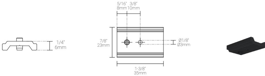
**1CT Track** | 60W driver for 1 to 6 8W fixtures. All 1CT fixtures comes with ECN0-1C16001-BK Track Adapter
