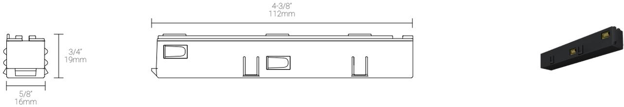
**1CT Track** | 60W driver for 1 to 6 8W fixtures. All 1CT fixtures comes with ECN0-1C16001-BK Track Adapter
